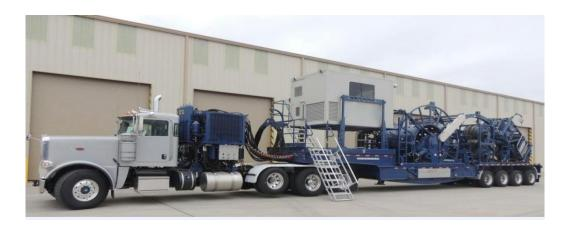
This Truck Mounted Coiled Tubing Unit (CTU) Hydra Rig 480, which will have the capability of working with Coiled Tubing Strings of up to 1-1/2" diameter, used for:
